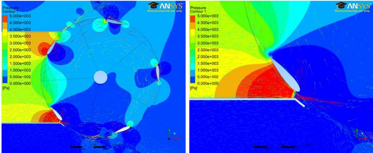
(a) Whole of the runner (b) Detail around right edge of the nozzle
