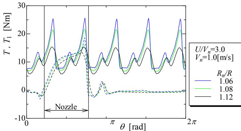
**Fig. 8** Torque fluctuation for one revolution of runner
