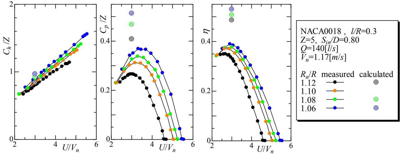
**Fig. 7** Influence of nozzle gap on turbine performance (symmetry gap with  $R_n=R_{na}=R_{nb}$ )
