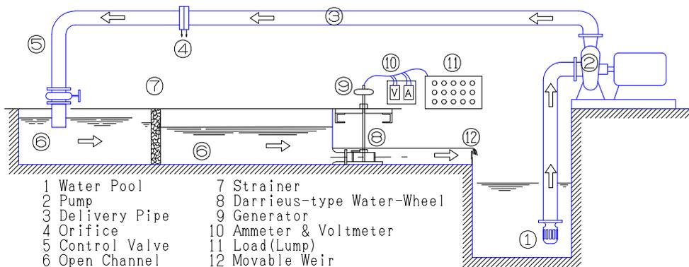
Fig. 5 Schematic view of experimental setup
