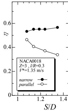
Fig. 4 Turbine efficiency against width of turbine casing walls
