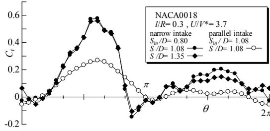
Fig. 3 Time variations of torque in one rotation of one Darrieus blade
