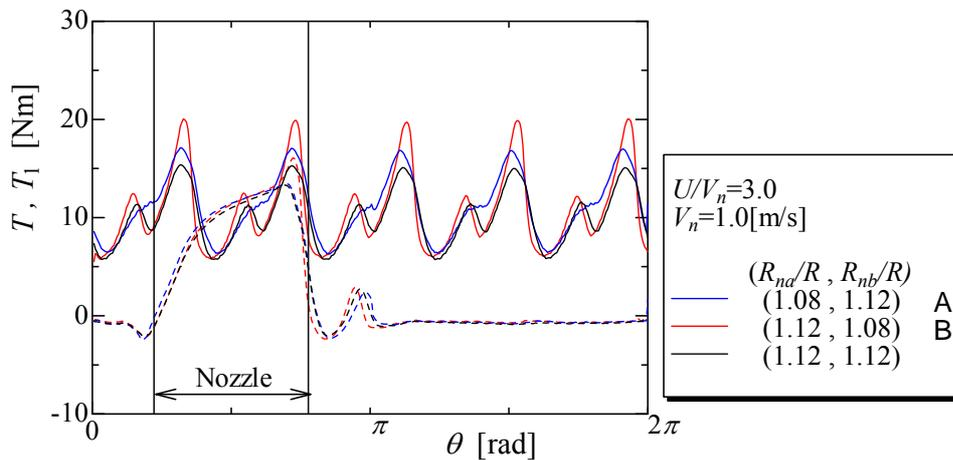
Fig. 12 Torque fluctuation for one revolution of runner
