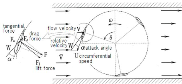
Fig. 2 Working principle of Darrieus turbine
