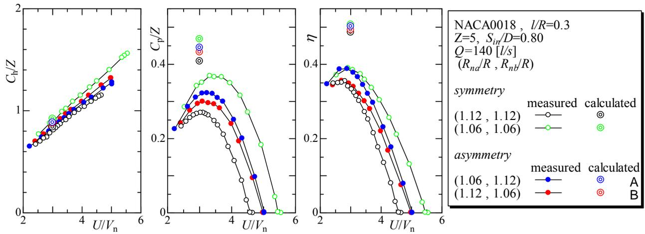
Fig. 11 Influence of nozzle gap on turbine performance (asymmetry gap)
