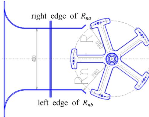
**Fig. 6** Arrangement of runner and original inlet nozzle
