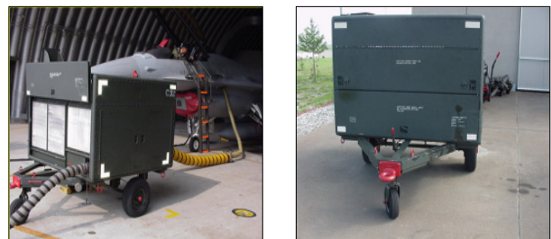
<Figure 6> Forming an Air Cooler to Fill Air Into an Aircraft
