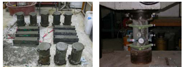
(a) Specimens for test (b) Compressive strength test
