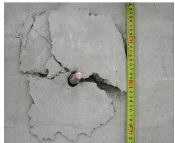
Fig. 4 Failure Mode for Embedment Depth
