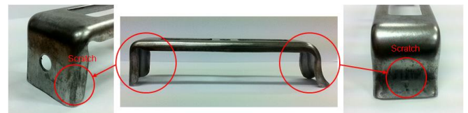
Fig.12 Scratch inferiorities during the stamping process of the bracket part
