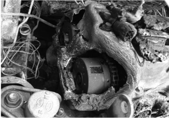
**Fig. 4.** Fire example burned plastic pet bottle on engine exhaust manifold part.
