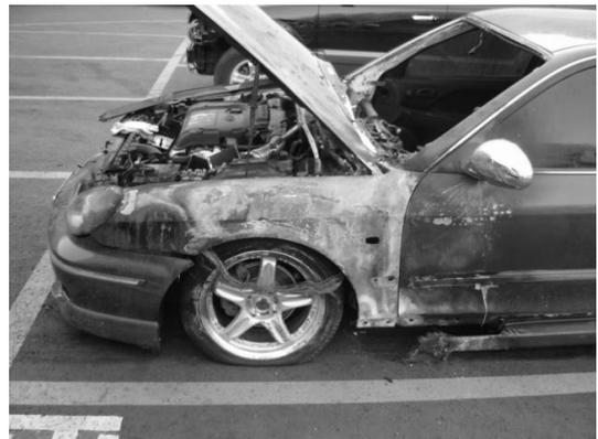
Fig. 2. Fire example by intake and exhaust system tuning.
