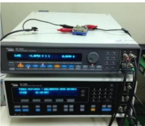
Fig. 6. Discharge test of zinc-air battery bolt cell
