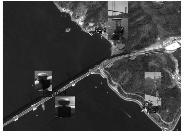
Fig. 2. Layout of GPS Campaign for Machang Grand Bridge
