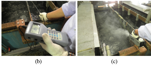
[Fig. 3] Measuring figure (a)Sampling point for capture velocity and HCl concentration (b)Hot wire anemometer (c)Fog machine
