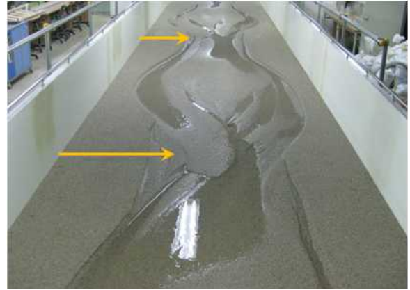
Fig. 1. Sediments Bars in the Channel with Periodic Variable Width (Jang, 2013): Arrows Indicate the Locations of Flow Concentration
