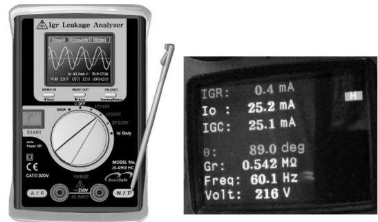
a) Instrument for analysis on leakage component
