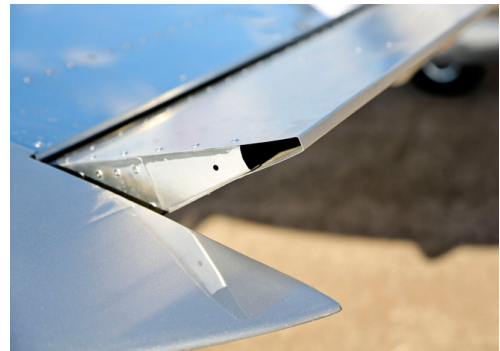
Fig. 1 Wing with finite trailing edge thickness
