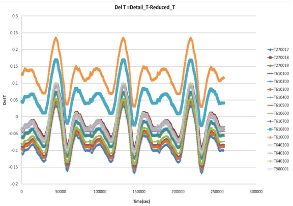
Fig. 17 Temperature difference between detailed model and reduced model vs. orbit time(24 hours)
