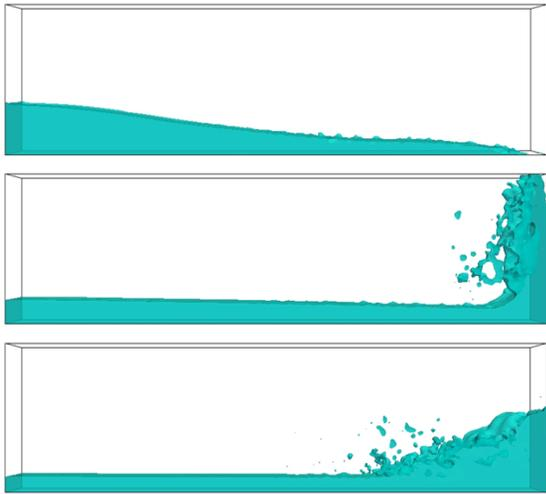
Fig. 11 Snapshot of the dam-breaking simulation at  $T=3$ (top),  $T=5$ (middle) and  $T=7$ (bottom). Where  $T$  is nondimensional time expressed at equation (41)
