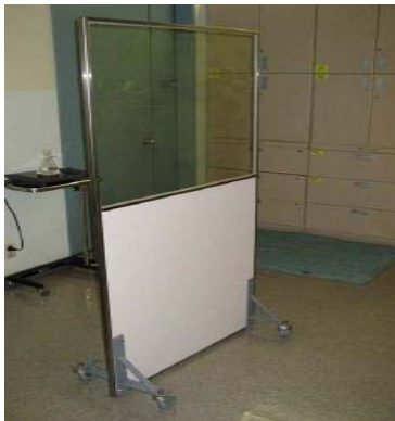
Fig. 2. Mobile lead protection.
