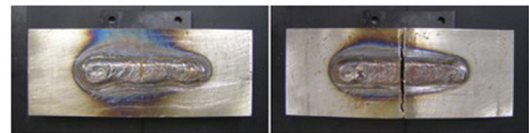
Fig. 7 Drop weight test results and images of test samples
