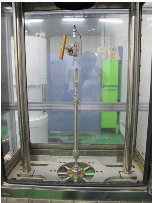
Fig. 6 An installed tube specimen.
