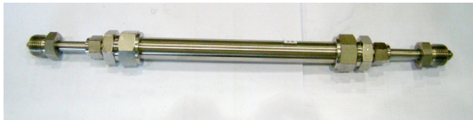
Fig. 5 Assembled tube specimen.
