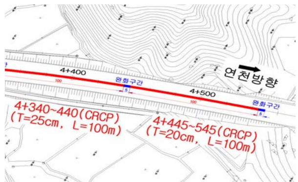
Fig. 4 Location of CRCP Construction at HoeCheon-SangPai Region (STA 4+340-545)
