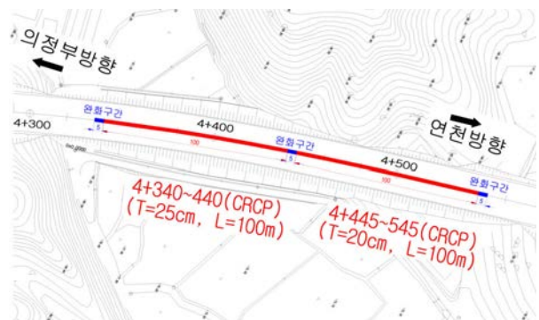
Fig. 1 Location of CRCP Construction at Hoecheon-Sangpai Region (STA 4+340-545)
