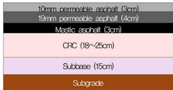
Fig. 1 Composite Pavement Layer Composition
