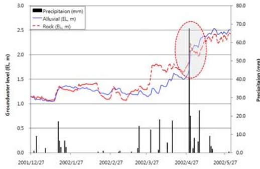
Fig. 8. Daily hydrograph of groundwater level's change at the national groundwater monitoring well.
