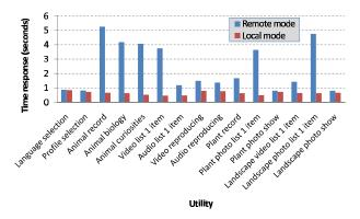
Fig. 8. Time response comparison local vs. remote mode, for the different views.
