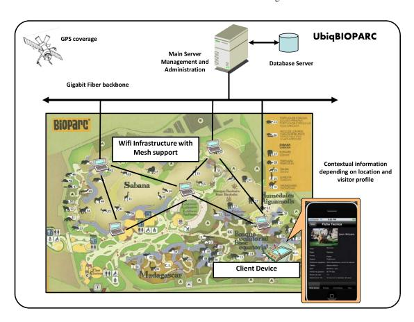
Fig. 2. UbiqBIOPARC System Architecture.
