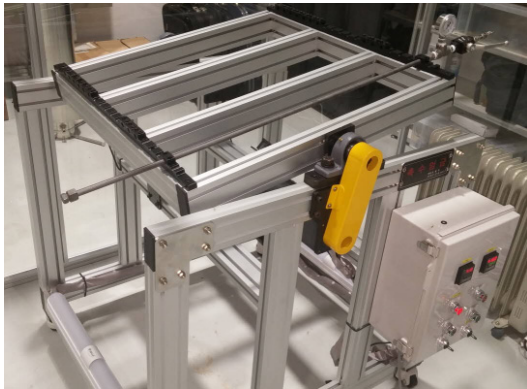
[Fig. 3] Photograph of swing system for mixing test fluid inside specimen with moving specimen as clock and counter-clockwise alternately
