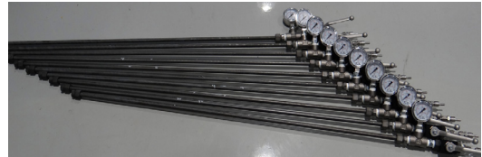
[Fig. 2] Photograph of test specimen with installation of plug fitting, pressure gauge, and on/off valve
