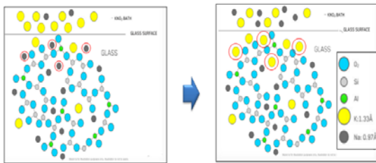
Fig. 2 Ion stuffing of sodium ions and potassium ions 7)
