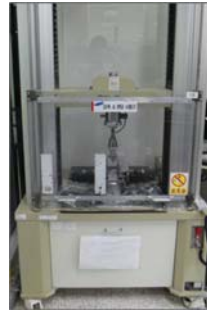
Fig. 6 3-Point bending tester 10)
