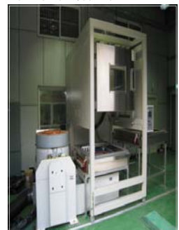
Fig. 9 Photographs in setting the jig and the shaker
