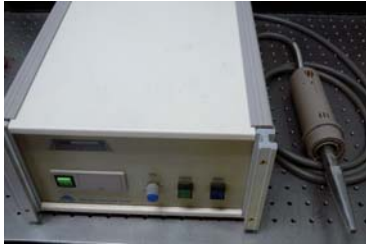
Fig. 5 Heating system using ultrasound excitation
