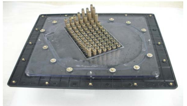
Fig. 4. Probe array disposition in the right SAM phantom.
