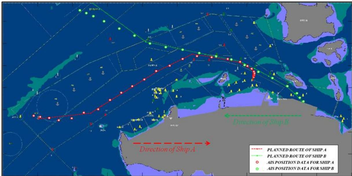
Figure 8. Ships' planned routes with position data.
