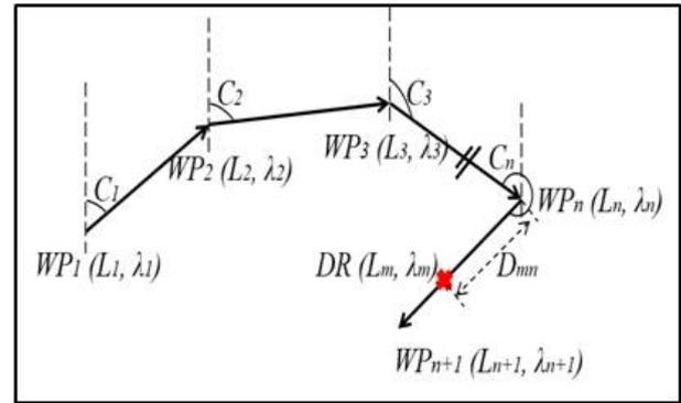
Figure 3. Proposed method of dead reckoning (DR) position calculation [11, 12].
