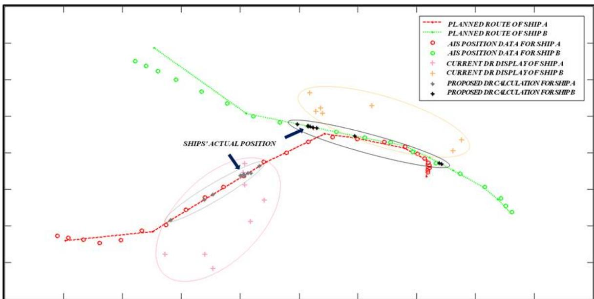
Figure 9. Comparison between traditional and proposed dead reckoning positions.
