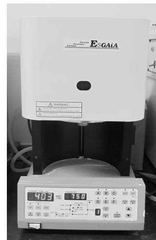
Fig. 2. Porcelain build-up furnace
