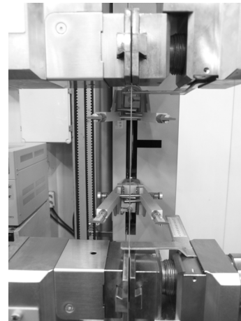
Fig. 3. Universal testing machine of tensile test
