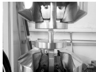
Fig. 2. Schematic diagram of the compression test setup on UTM
