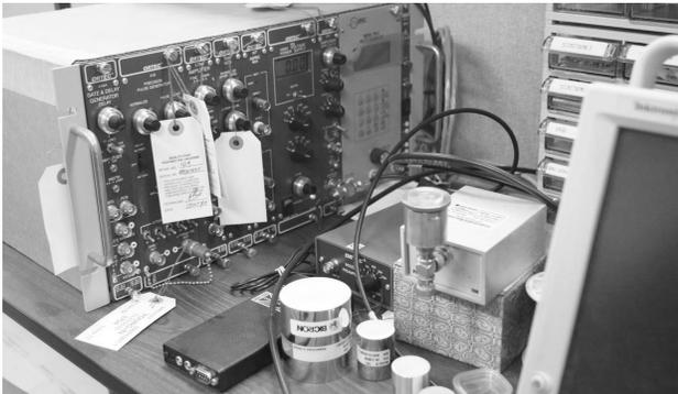
**Fig. 3** Photograph of a pulse height spectra measurement system. Full system consists of detector holder(eV product), preamplifier(eV product), shaping amplifier(ORTEC), and multi-channel analyzer(ORTEC)
