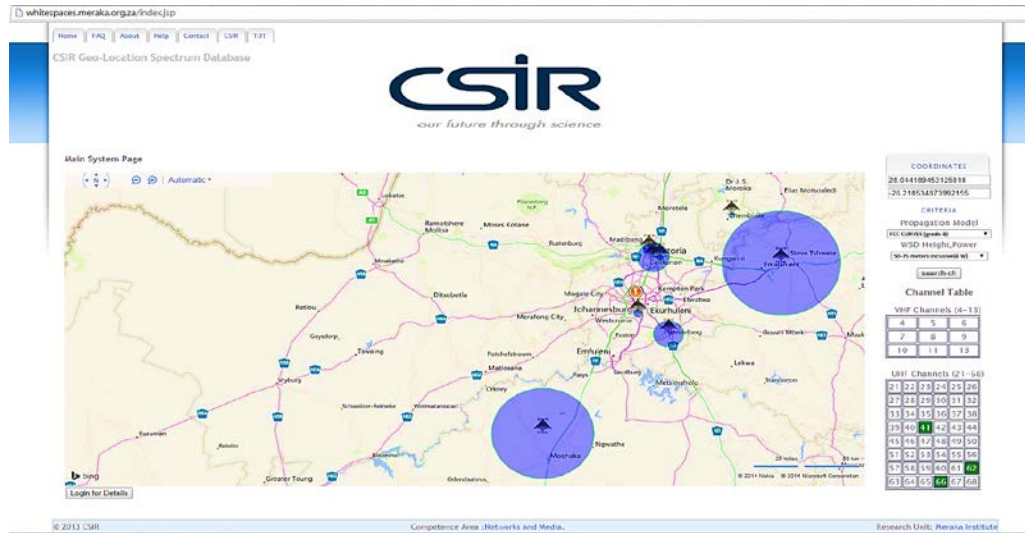
Fig. 9. CSIR-Meraka GL-WSDB using FCC-Curves wave propagation model showing 3 available channels (UHF channels 41, 62 and 66) for a 4 W fixed WSD with antenna HAAT of 50 m to 75 m in Johannesburg area, South Africa [38].
