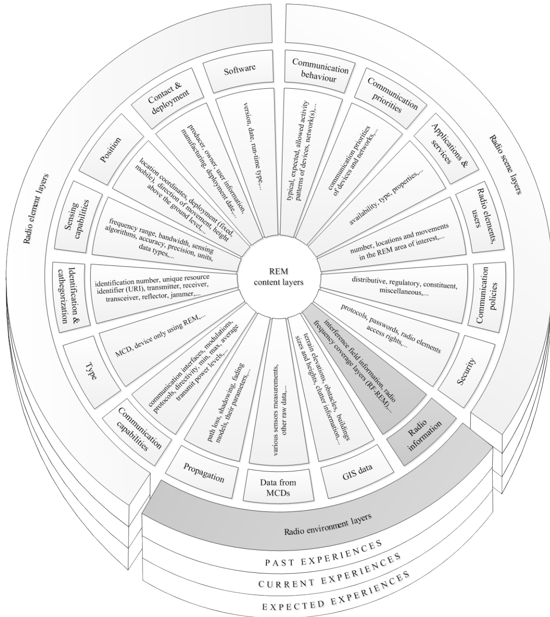
Fig. 2. The main content categories of the REM storage divided into layers and sub-layers.
