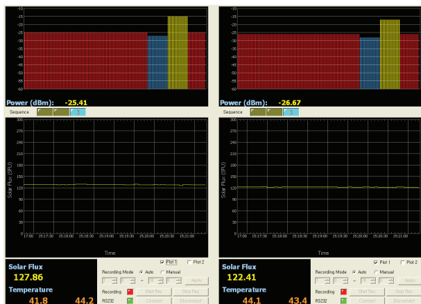
Figure 3. Graphical user interface of the program installed on the local PC. The data sets obtained by the two receivers are displayed separately in the left and right panels. The two top panels show the measured powers, in which blue, yellow, and red vertical bars represent the powers of ambient load, noise source, and sun, respectively.
