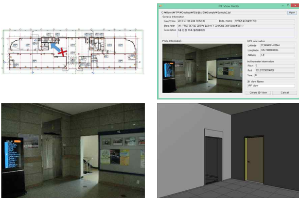
Figure 16. An example of extracting the position of a virtual camera from the vector photo information (lobby)
