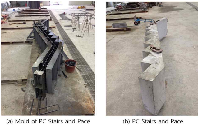
Figure 12. Integrated PC Stairs and pace
