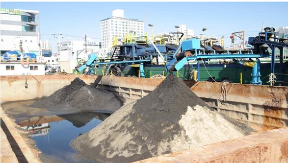
Figure 2. Particle size classification of dredged sea soil
