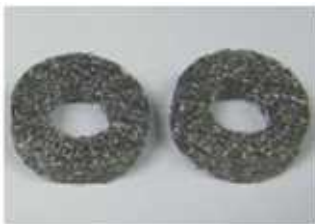
Fig. 2. Configuration of Pseudoelastic SMA Mesh Washer[5]
