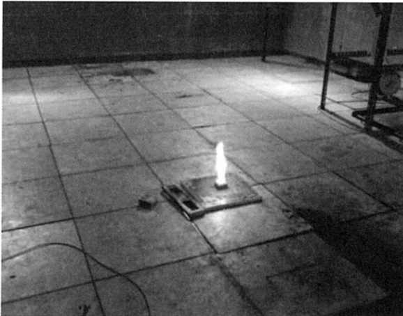
Fig 2. Photo of fire source – N Heptane pan
