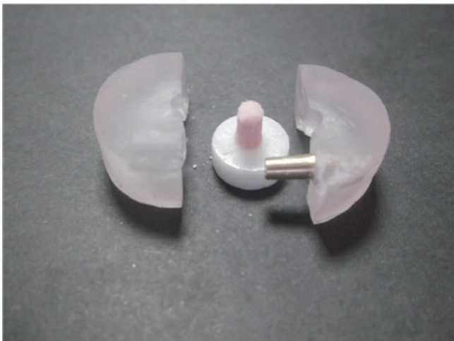
Fig. 1. Veneer ceramic fabrication using a specially designed split mold.
