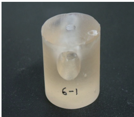
Fig. 4. Specimen of Group 5 (15% contact, 2 mm upper contact height).
