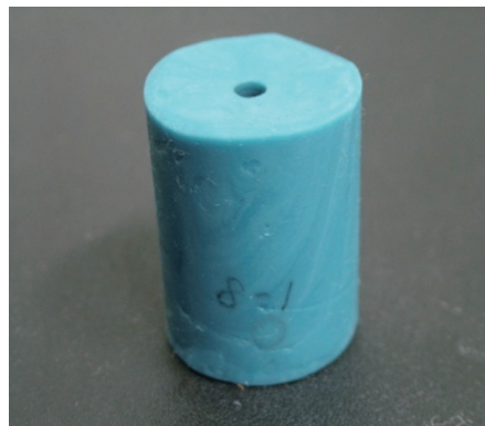
Fig. 5. Specimen of Group 7 (100% contact, impression putty block).
