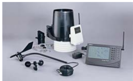
Figure 3: Parts of Weather Station [5]
