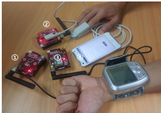
[Fig. 7] Picture of smart phone measuring DI(Dementia Index) from HRV and SpO 2 sensors
