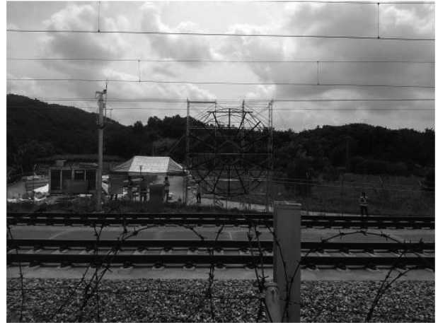
Fig. 7 Microphone array system
