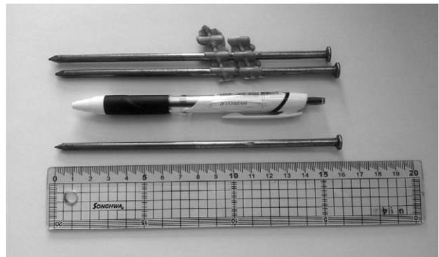
**Fig. 3.** Nail 160 mm × 4 mm, Nailhead diameter 7 mm
