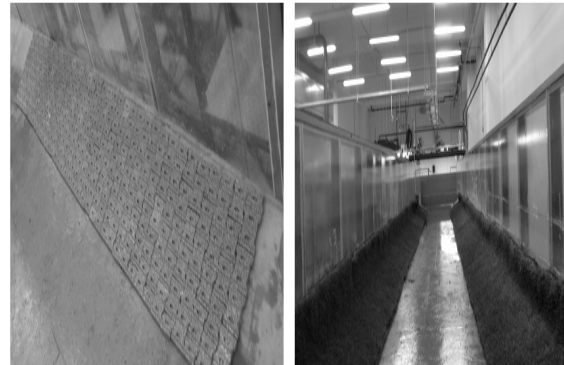
Fig. 12. Scale model block and vegetation installation
