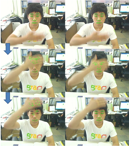
Fig. 4. Reinitialization of facial features after partial occlusions
