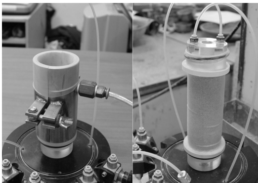
Fig. 1. Scenes of Triaxial apparatus test
