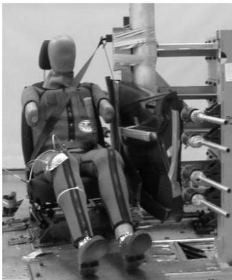
Fig. 7 vehicle to sled validation test using WorldSID
